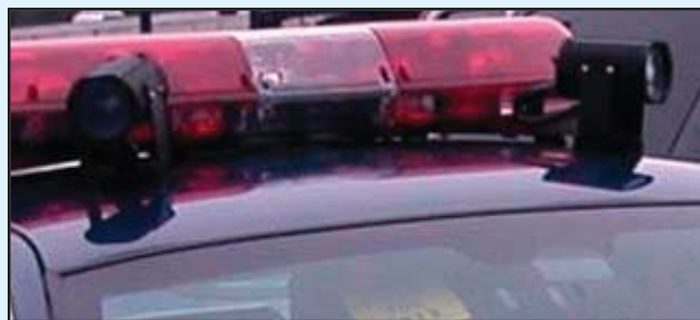
LPR unit installed onto cruiser's light bar.
