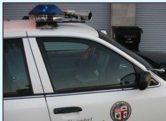
LPR unit installed onto cruiser's light bar.
